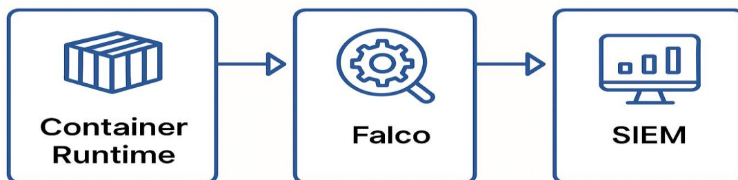
Figure 4: Sample Falco Detection Flow from Container Runtime to SIEM Alert
